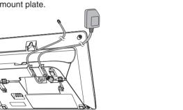
2. Press down on the tabs on the wall mount it from tabletop orientation. Rotate the wall and then push it into the telephone base until
