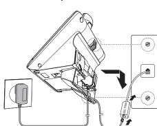
Unplug the telephone line cord (or the DSL filter) from the telephone wall jack. Unplug the power adapter from the electrical outlet. Slide the wall mount bracket up and remove it from
